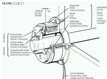
Note: The friction surfaces must be kept completely free of any lubricant or grease.
